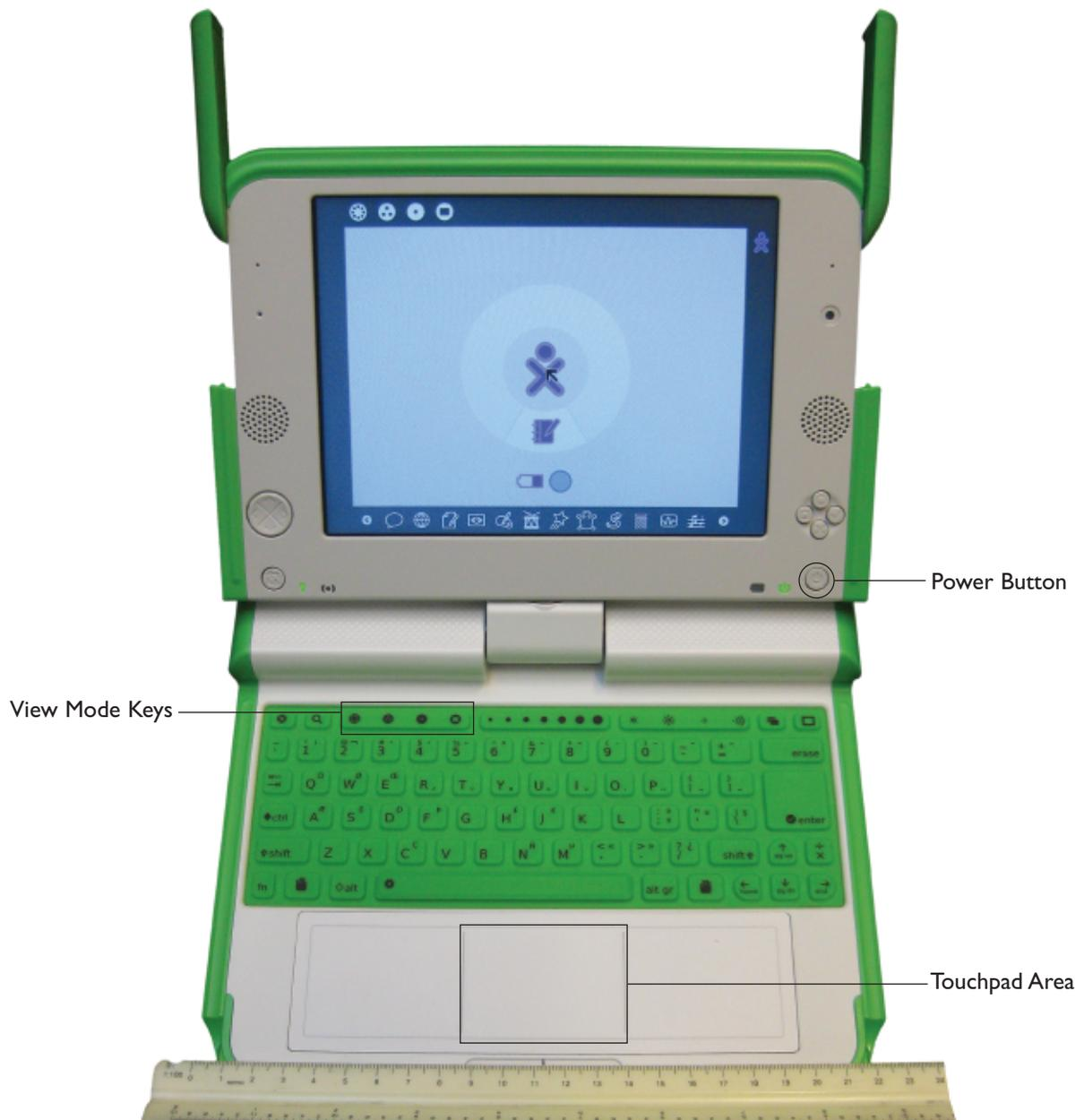
Figure 1. A picture of the XO laptop highlighting various parts of the machine. A ruler at the bottom provides scale.
